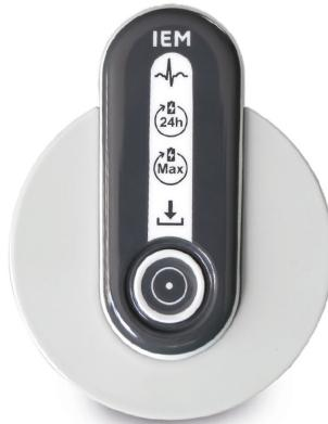
The device's LEDs provide clear indications of the charging process. While the battery charge is insufficient for a 24-hour recording, the 24h-LED will blink, and the Max-LED will remain off. Once the charge reaches a sufficient level for a 24-hour recording, the 24h-LED will stay constantly on, and the Max-LED will begin blinking, indicating that the battery is continuing to charge.
