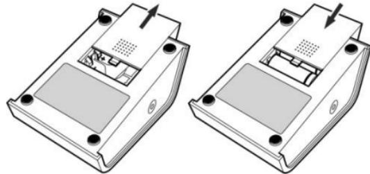
Fig. 4: Opening the battery cover
