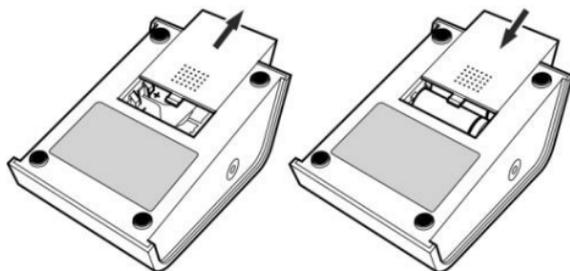
Fig. 4: Opening the battery cover
