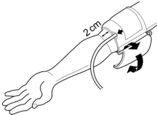
Fig. 8: Correct position of blood pressure cuff
